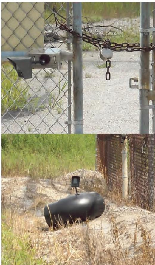
← This MotionViewer was mounted directly on the front gate. Because they are “unplugged” and require no AC power, they can be installed where they are most effective.
